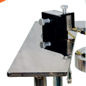
Solid station frame with built-in vibration-isolations.
