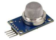
MQ-135 Air Quality & Hazardous Gas Sensor
